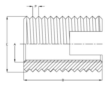
Female thread A = M22 Length B = 30 Male thread E = 26.0 Min hole depth blind hole = 36
